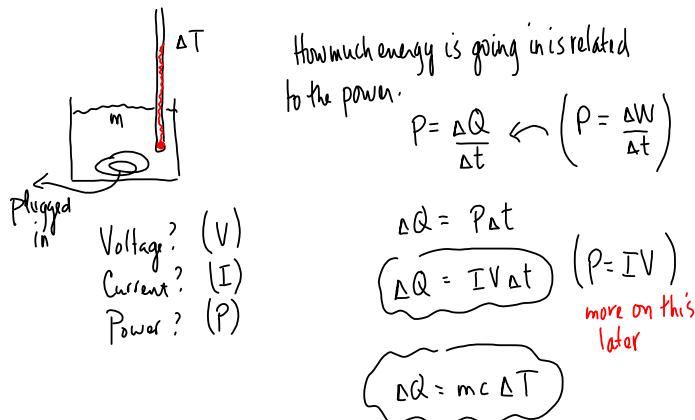
$$\begin{aligned} IV \Delta t &= mc \Delta T \\ C &= \frac{IV \Delta t}{m \Delta T} \end{aligned}$$
